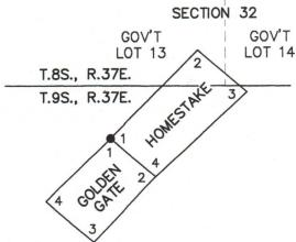
ORIGINAL DESCRIPTION: A fir post 4 ft. long, 5 ins square set 18 ins in the ground, surrounded with a mound of earth scribed Homestake 1-514 and Golden Gate-1-514 Identical with location S.W. cor. post. From which
