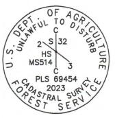
Placed a plastic-encased magnet beneath the base of the aluminum pipe. Used a total station to measure the reference points. Set an aluminum guard post North, 3.8 ft., with USFS 54-2 and 54-9 signs attached, and another N.49°W., 2.5 ft., with USFS 54-2 sign attached. See associated Map of Survey dated October 17, 2023 for survey-related information.
