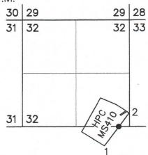
**ORIGINAL DESCRIPTION:** Set a  $2\frac{1}{2}$ " aluminum cap on 2" aluminum pipe 30 ins long 25 ins in ground with 5 ins proj. out of ground with surrounding rock mound and 6 ft steel fence post alongside with sign 54-9 attached.
