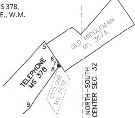
**ORIGINAL DESCRIPTION:** Set a white fir post 4 ins. square  $4\frac{1}{2}$  ft. long 18 inches in the ground with a mound of earth around it marked TEL C7- 378
