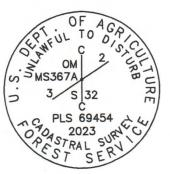
Placed a plastic-encased magnet beneath the base of the aluminum pipe. Used RTK GPS to measure the reference points. Set an aluminum guard post South, 6 ft., with USFS 54-2 sign attached, and another S.56°W., 6 ft., with USFS 54-2 and 54-9 signs attached. See associated Map of Survey dated October 17, 2023 for survey-related information.
