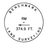
► A 5/8"x30" iron pin, set on the north side of a rock gabion gate support, bears S.31°48'45"E., 400.78ft. with attached aluminum cap marked as shown:
