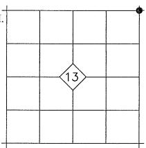
**ORIGINAL DESCRIPTION:** Set Basalt stone 14X10X8 ins, 10 ins in the ground for cor to secs 7, 12, 13 and 18 and marked with 2 notches on N and 4 notches on South edges and raised a mound of stone alongside. Pits impracticable.
