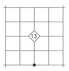
**ORIGINAL DESCRIPTION:** Set Basalt stone 18x12x7 ins, 12 ins in the ground for 1/4 Sec. Cor marked 1/4 on N face and raised a mound of stone alongside.
