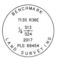
Used RTK GPS to measure the reference points. Bearings are based on Geodetic North determined by GPS observation at the SW Corner Section 13, T.13S., R.36E.
