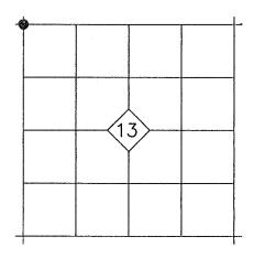
**ORIGINAL DESCRIPTION:** Set Basalt stone 24x12x6 ins, 18 ins in the ground for Cor to secs 11, 12, 13 and 14 marked with 4 notches on the S and 1 notch on E edges and raised a mound of stone alongside. Pits impracticable.
