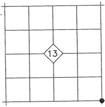
**ORIGINAL DESCRIPTION:** Set Basalt stone 16X14X5 ins, 11 ins in the ground for cor to secs 13, 18, 19 and 24 and marked with 3 notches on N and S edges and raised a mound of stone alongside. Pits impracticable.
