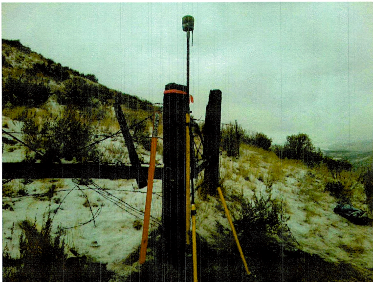
B . Measuring the established section corner.
