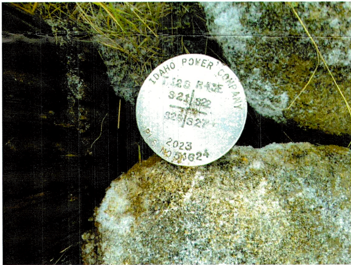
A . Set 30 X 2 1/2 in. aluminum post at the corner point alongside fence corner.
