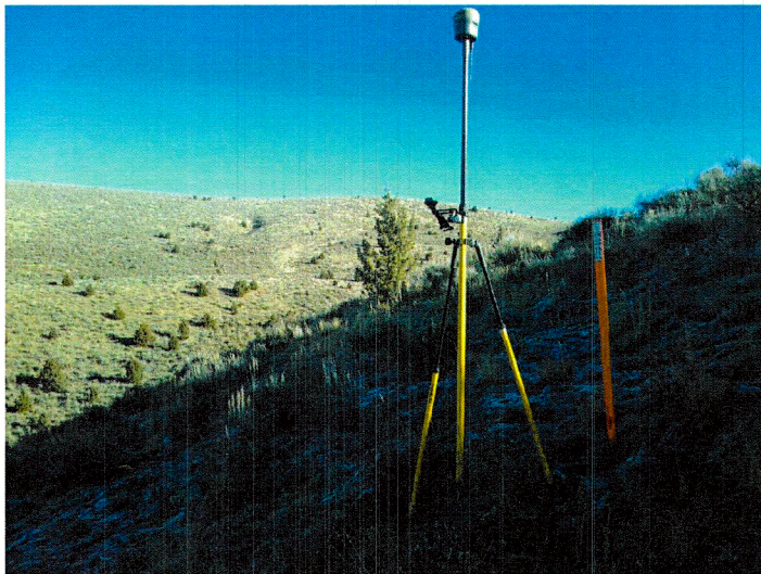
C . Measuring the 1/4 section corner.
