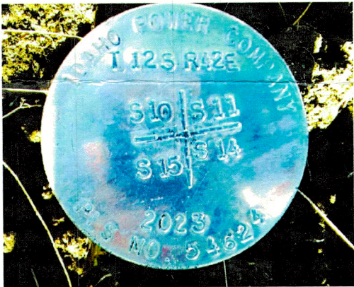
B. 30 x 2 1/2 ins. aluminum post set at the corner point
