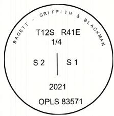
I used a Leica GS14 with RTK in the establishment of the new bearing objects. Distances and bearings are to the center of the aluminum caps.
