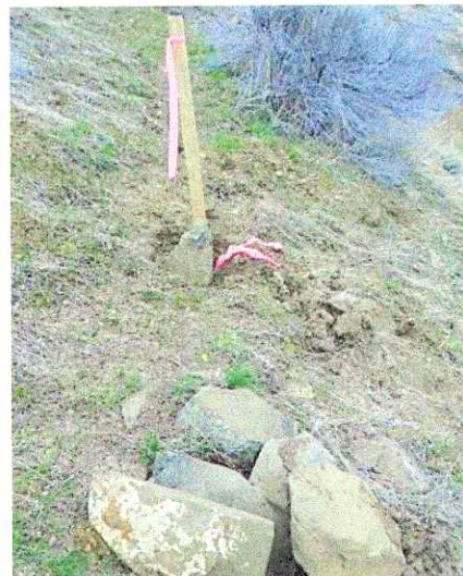
Looking south, the quarter corner stone and original mound is in place as described in GLO notes.
