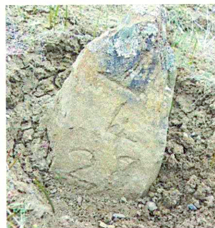
After exposing the north face of the cornerstone, the markings 1/4 28 are clearly visible.
