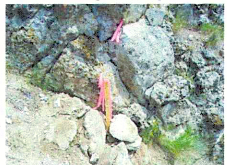
Railroad spike and PK spike bearing objects, as well as the 1/4 corner location are shown at the base of the conglomerate rock bluff.
