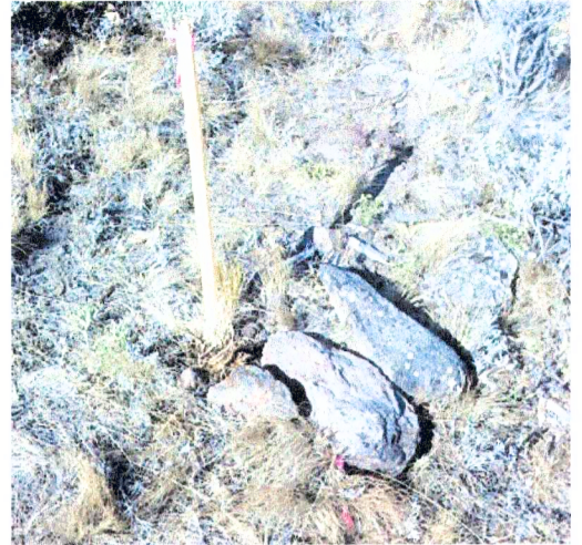
Found stone 14" x 12" x 6" and mound of stone nearly fitting the description in the GLO field notes of Henry Meldrum.
