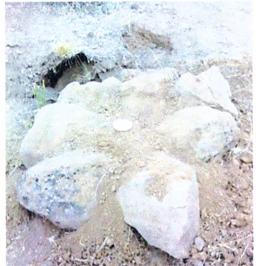
Set brass cap monument to within 8" of the surface in a mound of stone 3 feet at base around monument. Original stone is buried on the North side of monument.
