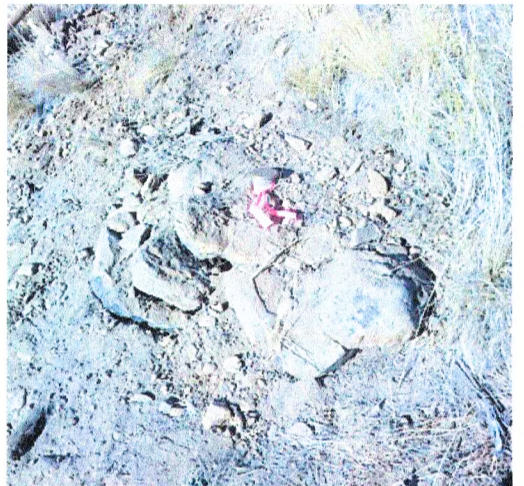
Set brass cap monument to within 8" of the surface in a mound of stone 3 feet at base around monument. Original stone is buried on the North side of monument.
