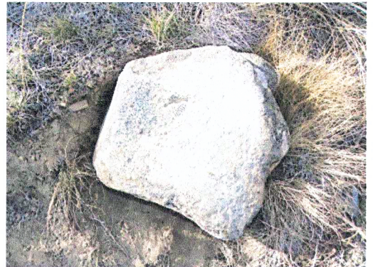
Found a Basalt stone 12"x 10"x 6" as described in Reuben R. Leigh's field notes of his GLO survey. The markings 1/4 are barely visible in the top center part of the stone.
