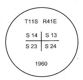
I use a steel tape and magnetic compass in the establishment of the bearing trees. I use 16° East declination. Distances are to a 60d spike in the right hand side of the root crown of the trees. Bearings are to a brass washer marked OPLS 83571 in the lower blaze.
