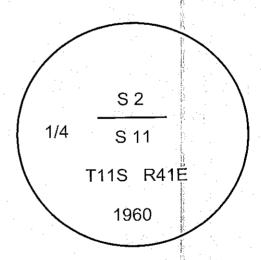
I use a steel tape and magnetic compass in the establishment of the new bearing trees. I use 16° East declination. Distances are to a 60d spike in the right hand side of the root crown Bearings are to a brass washer marked OPLS 83571 in the lower BT blaze.
