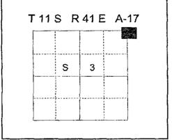
Set an iron post, 28 ins. Long, 2 ½ ins. diam., 24 ins. in the ground with brass cap. A mound of stone, 2 ft. diam., 4 th. High, used as a fence cradle, bears South, 2 lks. dist.
