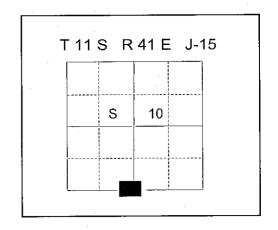
Set an iron post, 28 ins. Long, 2 ½ ins. diam., 24 ins. in the ground, with brass cap. From which:
