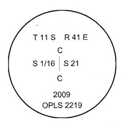
I used a steel tape and magnetic compass in the establishment of the bearing trees. I used 18° East declination. I attached a brass washer marked OPLS 2219 to the BT blaze. The distance is to a 60d spike driven into the root crown at the right side of the bearing trees.
