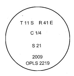
I used a steel tape and magnetic compass in the establishment of the bearing trees. I used 18° East declination. I attached a brass washer marked OPLS 2219 to the BT blaze. The distance is to a 60d spike driven into the root crown at the right side of the new bearing tree.
