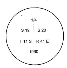
I used a steel tape and magnetic compass in the establishment of the new bearing tree. I used 18° East I attached a brass washer marked OPLS declination. 2219 to the BT blaze. The distance is to a 60d spike driven into the root crown at the right side of the new bearing trees. Bearings and distances to found accessories are to the center of the tree.
