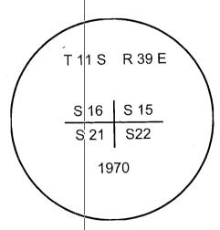
I used a steel tape and magnetic compass in the establishment of the accessories. Declination used was 16° East. Bearings and distances are taken to the center of the tree. On the new bearing trees, distances are taken to a 60d spike in the right hand side of the root crown.
