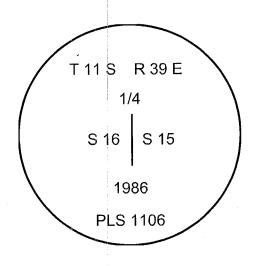
I used a steel tape and magnetic compass in the establishment of the accessories. Declination used was 16° East. Bearings and distances are taken to the center of the tree. On the new bearing tree, distance is taken to a 60d spike in the right hand side of the root crown.
