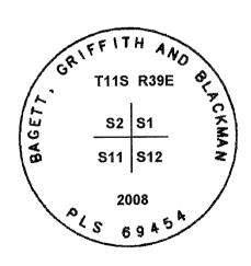
Raised a mound of stone 3 ft. base to top of cap. Used RTK GPS to measure accessories.
