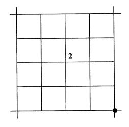
ORIGINAL DESCRIPTION: Set a basalt stone 16X12X12 10 in. deep for cor. to Sec. 1,2, 11, 12 marked with 5 notches to S. 1 notch on E. edges raised Md stone alongside.
