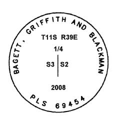
Raised a mound of stone 3 ft. base to top of cap. Used RTK GPS to measure accessories. Distances to BT's measured with a steel tape to a 50d nail driven in the side-center at the root crown of the trees. Attached a BT tags to the trees.
