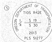
AT POSITION BY PROPORTIONATE MEASUREMENT, THERE BEING NO REMAINING EVIDENCE OF THE ORIGINAL CORNER: SET 2 1/2 INS. DIAM. ALUM. POST, BURIED 21 INS. IN THE GROUND, WITH 3 1/4 INS. DIAM. ALUM. CAP MARKED AS SHOWN, WITH CLEAR DEEP-1 MAGNET AT BASE AND STONE MOUND SURROUNDING, A GALV. IRON POST SET WEST 1.5 FT., FROM WHICH:
