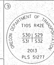
AT POSITION OF FOUND STONE SET BY BAKER COUNTY SURVEYOR IRA HOFFMAN, STONE IS 12 INS. X 15 INS. X 21 INS., WITH 5 BARS ON ONE FACE, LYING ON SIDE IN OLD FENCELINE AT SOUTH RIGHT OF WAY LINE OF RAILROAD, SET 2 1/2 INS. DIAM. ALUM. POST, BURIED 20 INS. IN THE GROUND, WITH 3 1/4 INS. DIAM. ALUM. CAP MARKED AS SHOWN, WITH CLEAR DEEP-1 MAGNET AT BASE AND ROCK COLLAR, ORIGINAL STONE PLACED ALONGSIDE, FROM WHICH:
