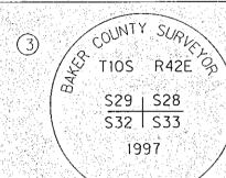
FOUND A 2 1/2 IN. DIAM. BRASS CAP ON A 1 1/4 IN. DIAM. GALV. IRON PIPE, UP 10 INS. IN A MOUND OF STONE, AT SOUTHEAST SIDE OF FENCE CORNER, MARKED AS SHOWN. SHOWN ON COUNTY SURVEY NO. 10-42-1, SHEET 4, MONUMENT RECORD NO. CP#43.
