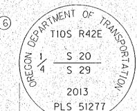
AT POSITION OF FOUND QUARTZ STONE, 8" X 9" X 12" LYING ON LONG SIDE, MARKED 1/4 ON ONE FACE, SET: 2 1/2 INS. DIAM. ALUM. POST, BURIED 19 INS. IN THE GROUND, WITH 3 1/4 INS. DIAM. ALUM. CAP MARKED AS SHOWN, WITH CLEAR DEEP-I MAGNET AT BASE AND STONE MOUND, ORIGINAL STONE PLACED ALONGSIDE, A T-POST PLACED ALONGSIDE EAST, FROM WHICH:
