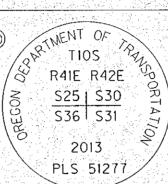
AT POSITION OF FOUND STONE, 8" X 9" X 22" (10" EXPOSED) FIRMLY SET WITH 6 NOTCHES ON WEST, I NOTCHES ON SOUTH AND 3 DISTINCT NOTCHES ON NORTH, T-POST SET BY UNKNOWN PARTY BEARS WEST IFT. SET: 2 1/2 INS. DIAM. ALUM. POST, BURIED 22 INS. IN THE GROUND, WITH 3 1/4 INS. DIAM. ALUM. CAP MARKED AS SHOWN, WITH CLEAR DEEP-I MAGNET AT BASE AND STONE MOUND, ORIGINAL STONE PLACED ALONGSIDE, FROM WHICH:
