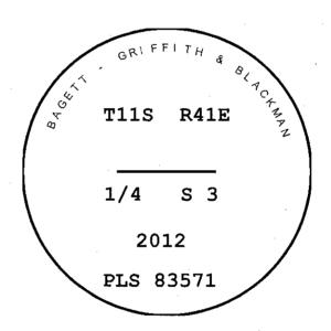
I used a Leica 1200 RTK GPS in the establishment of the iron pin accessories. Basis of bearings is as per survey for Gallatin NE Oregon Land and Timber dated May 2012, as filed in the office of the Baker County Bearings and distances are to the center of Surveyor. the aluminum cap. Bearings to the bearing tree are established by magnetic compass and steel tape. Magnetic declination used was 16° East. Distance is to a 50d spike placed in the right hand side of the root crown.
