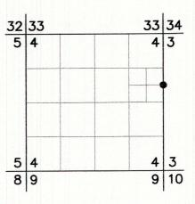
**ORIGINAL DESCRIPTION:** Survey No. 10-39-168 shows a 5/8" rebar with plastic cap marked "HANLEY ENGR. PLS 1817" set at the corner.
