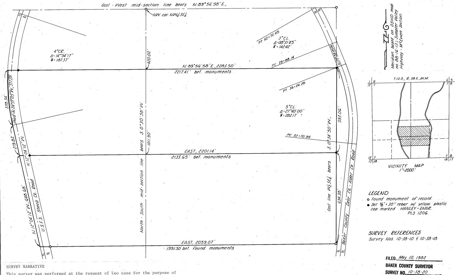
This survey was performed at the request of Leo case for the purpose of boundary monumentation and description preparation of that land shown on this map and located in the  $E^1_2SW^1_4$  and  $W^1_2SE^1_4$  of Section 7, T 10 S,
