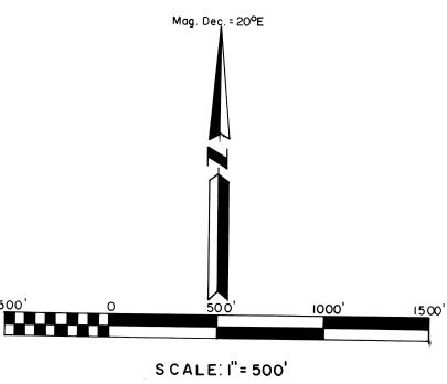
BASIS OF BEARINGS SOLAR OBSERVATION, WITH TRUE MERIDIAN ON LINE BETWEEN SEC. 30/29, T.IOS R.36E. MAGNETIC COMPASS IS NOT RELIABLE IN THIS AREA.
