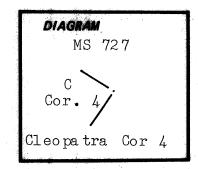
A 8" fir bears N4°W-4.9'. A 8" fir bears N65°E-10.3'. Both marked C-4-727 BT.
