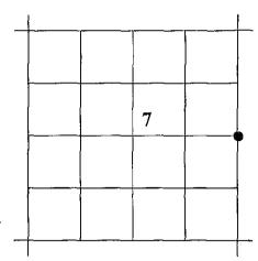
**ORIGINAL DESCRIPTION:** 40.00 Ridge course NW, Set basalt rock 12x10x6 ins, 8 inches in ground for 1/4 Sec corner, marked 1/4 on the West side, dug pits 18x18x12 ins, 5½ ft. dist N&S of stone and raised mound of earth 1½ ft high 3½ ft. base alongside
