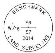
Used RTK GPS to measure the reference points. Bearings are based on Geodetic North obtained by GPS observation at the SW Corner Section 7, T.9S., R.41E.
