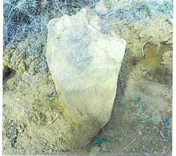
At this Quarter Corner location I found a very dimly double marked Basalt stone that measures 18"x 11"x 8"; the marked stone closely agreeing as described in W. B. Barr's field notes. Notice the very dim double 1/4 markings as I have lightly highlighted using a black lumber crayon to outline the marks.
