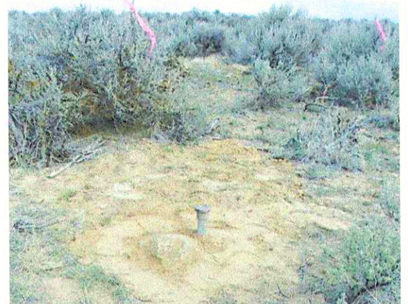
Buried monument to within 8 inches of the surface. Original stone was placed upside down with the tip above the surface on the North side of the Brass Cap. There are no other stone available in the general area of the monument.
