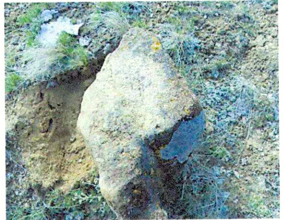
At this Quarter Corner location I found a marked Basalt stone that measures 20"x 12"x 10". The marked stone somewhat agreeing as described in W. B. Barr's field notes. Notice the markings 1/4 as I have highlighted using a black lumber crayon to out line the clearly visible chisel marks.
