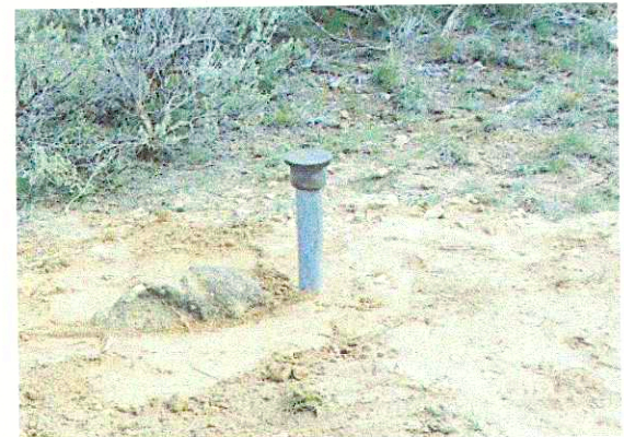
Buried monument to within 8 inches of the surface. Original stone was placed upside down with the tip above the surface on the North side of the Brass Cap. No other stone are available in the general area of this monument.
