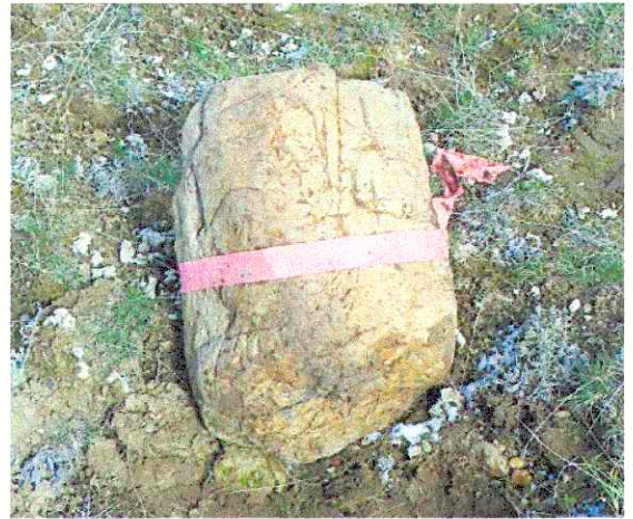
At this Quarter Corner location I found a marked Quartzite stone that measures 16"x 10"x 6". The marked stone somewhat agreeing as described in W. B. Barr's field notes. Notice the markings 1/4 as I have highlighted using a black lumber crayon to outline the clearly visible chisel marks.
