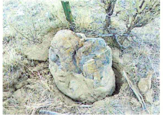
At this Section Corner location I found a marked Quartzite type stone that measures 14"x 9"x 6", somewhat agreeing as was described in W. B. Barr's field notes. Notice the markings 2 notches on the South and 2 notches on the East faces, as I have highlighted using black lumber crayon to outline the clearly visible chisel marks at the center face of the stone.
