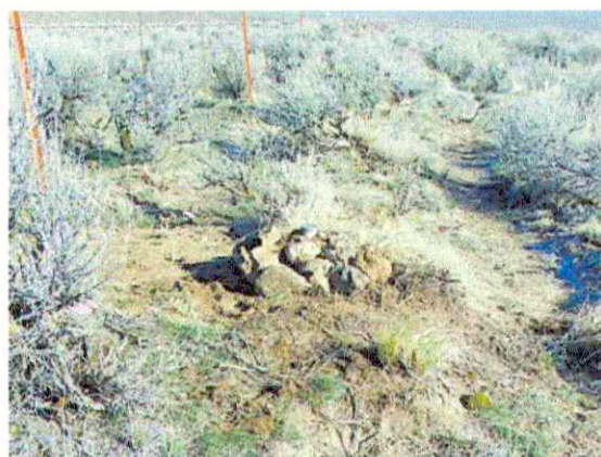
Brass cap and mound of stone as they appeared before covering the mound with soil to assist in protecting and stabilizing the mound. Notice The reference monument near the upper center of the photo as well as the existing North-South fence line located 5 feet to the West of the corner.
