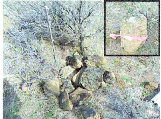
Found large mound of stone at section corner location. Insert photo shows stone measuring 15" x 10" x 7", closely fitting W. B. Barr's description of the stone he claimed to have set. Stone was found and recovered from the center of the large mound as if it was intentionally buried, possibly for protection.
