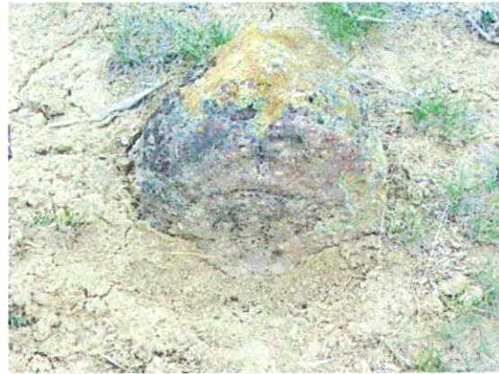
At this Quarter Corner location I found a marked Volcanic stone that measures 12"x 11"x 6". The marked stone agreeing closely as described in W. B. Barr's field notes. Notice the markings 1/4 as I have highlighted using a black lumber crayon to out line the clearly visible chisel marks.
