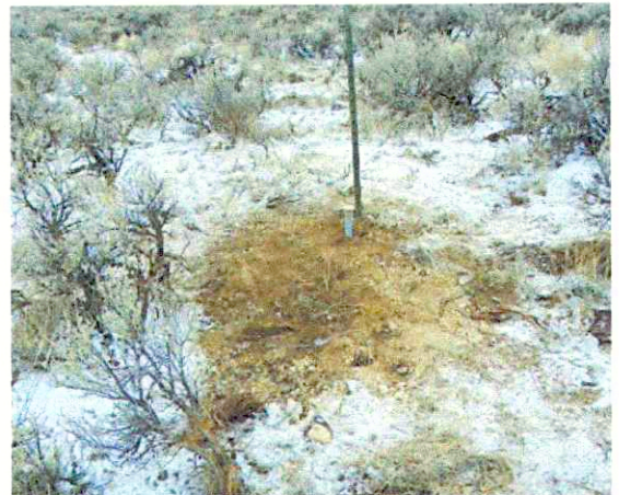
Buried monument to within 7 inches of the surface. Original stone was placed below the surface on the West side of the Brass Cap. No other stone was available in the area. I then reset the steel fence post alongside the monument to aid in locating the monument in the future. Notice the reference pin located in the background near the top center of photo.
