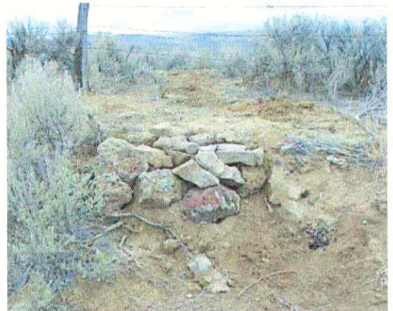
Brass cap and mound of stone as they appeared before covering the mound with soil to assist in protecting and stabilizing the mound. Notice the reference pin located to the North in the background near the top center of photo.
