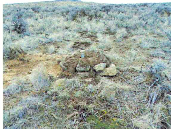
Brass cap and mound of stone as they appeared before covering the mound with soil to assist in protecting and stabilizing the mound. Notice the reference pin located in the background near the top center of photo.
