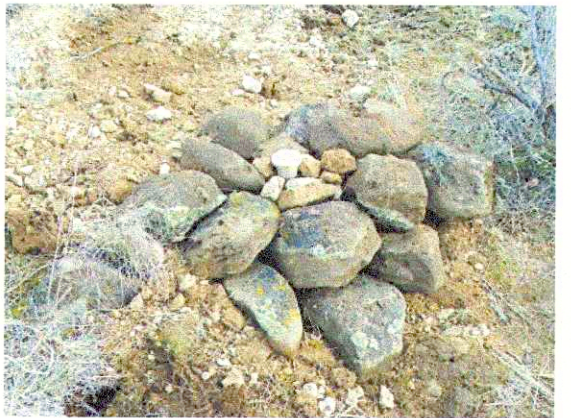
Brass cap and mound of stone as they appeared before covering the mound with soil to assist in protecting and stabilizing the mound. I then reset the steel fence post alongside the mound to aid in locating the monument.
