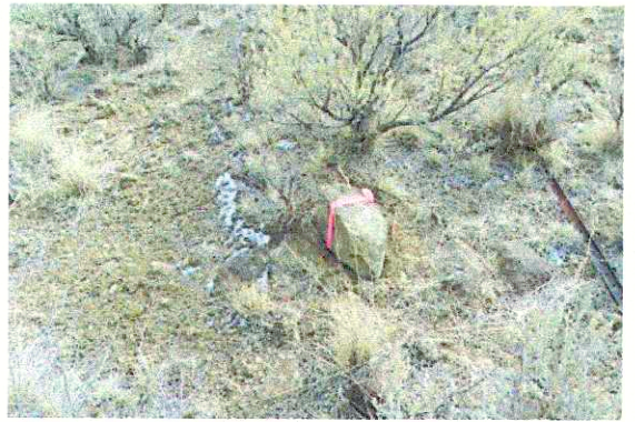
Found a stone closely fitting W. B. Barr's description of the stone he set. No visible markings can be identified on the stone. An additional mound of stone and a steel fence post are present at this corner location.
