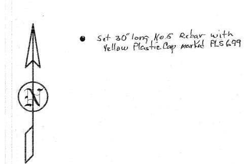
BASIS FOR BEARINGS GPS State Plane Coordinates
